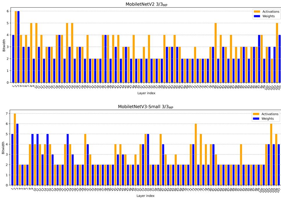
Figure 5: Final bitwidth allocation for MobileNetV2 and MobileNetV3-Small using QBitOpt with 3-bit average target bitwidth  $3/3_{MP}$ .
