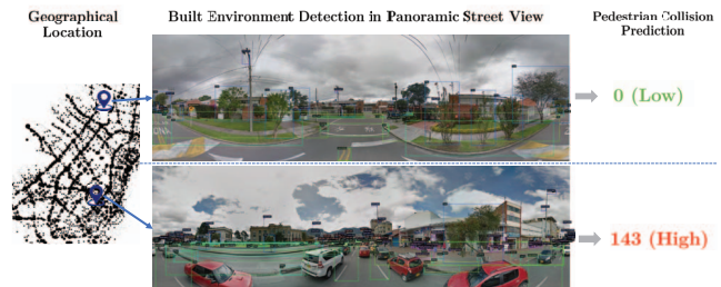
Figure 1: STRIDE . Given specific city coordinates (left) and the corresponding panoramic street view image (middle), we propose to predict the number of pedestrian collisions in those coordinates (right) by detecting built environment features (middle).
