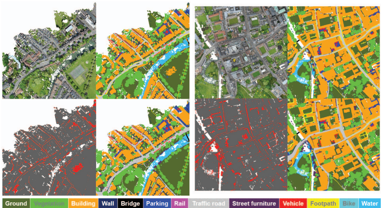
Figure 4. The qualitative result of two blocks in the validation set of SensatUrban [8]. In each figure, the top-left sub-figure is the aerial visualization of the original point cloud which covers a 400m \times 400m area. The top-right and bottom-right sub-figures are the predictions and ground truth respectively. Both of them follow the color bar at the bottom. The bottom-left sub-figure is an error map that presents the difference between the prediction and the ground truth.
