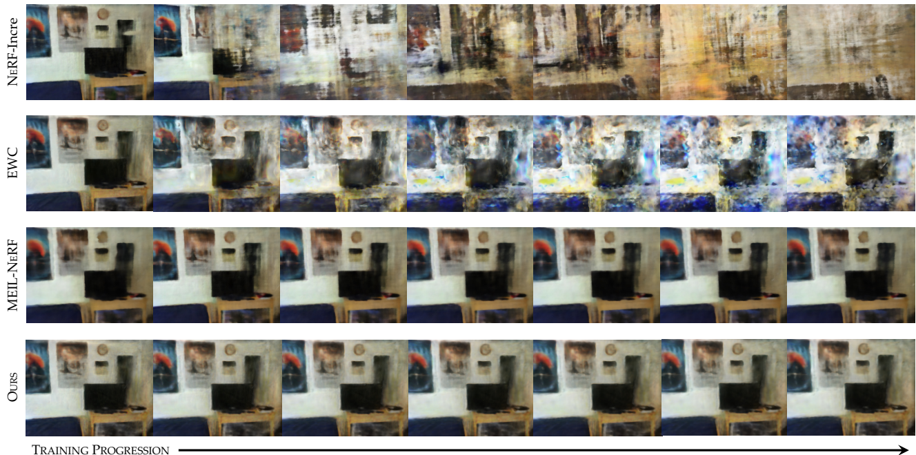
Figure 1. Reconstructed view of earlier task during different stages of training. Quantitative results shown in Figure 6 are obtained from evaluating PSNR of the right-most column.
