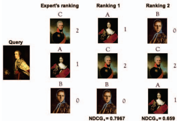
Figure 2. Calculated NDCG metrics for two rankings, expert’s ranking is the ranking with objects ranked in the most relevant order according to the expert’s criterion, 2, 1, 0 — the relevance scores rel_i in the ground truth ranking.
