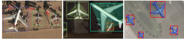
Figure 2. Three annotation styles within RarePlanes. The dataset features three annotation styles including: 'Bounding Box', 'Diamond Polygon', and 'Full Instance Segmentation' (synthetic only).
