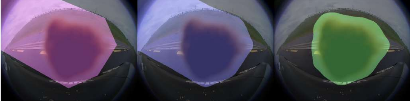
Figure 1: The problem of weak annotation labels and how generated data can help, presented on a testing image, which was not used during the training. The images come from the WoodScape Dataset . Left: original weak (polygonal) annotation; Note, that not only it is very coarse, but also prone to errors. Middle: semantic segmentation output, when trained on the weak annotation labels in a fully supervised manner. Right: the same semantic segmentation network output, however, in this case also the generated data were used. Note, how having precise annotation labels for the generated data help in refining the segmentation output.
