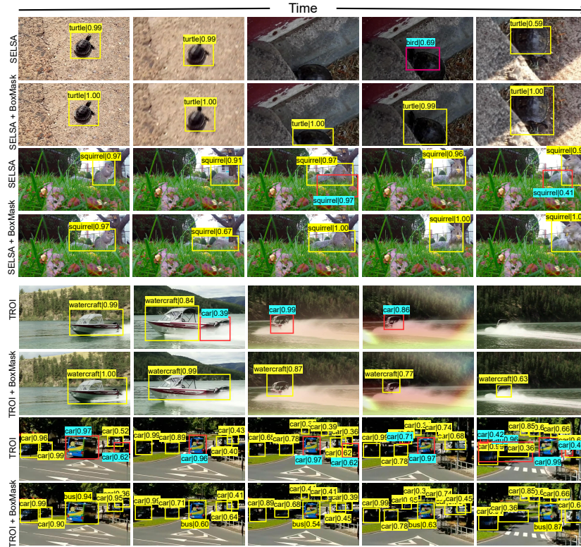
Figure 2. Qualitative analysis between existing methods without and with our BoxMask module on the validation set of the ImageNet VID dataset under different scenarios. With our BoxMask in SELSA [2], the detector removes false classification (turtle) and provides consistent results in case of rare poses and part-occlusions (top four rows). With the addition of our BoxMask module in TROI [1], the combination of temporal and semantic cues yields stable detections that are more robust to the motion blur/camera defocus and part-occlusions (last four rows). The illustration scheme is inspired by [4]. Best view it on the screen and zoom in.
