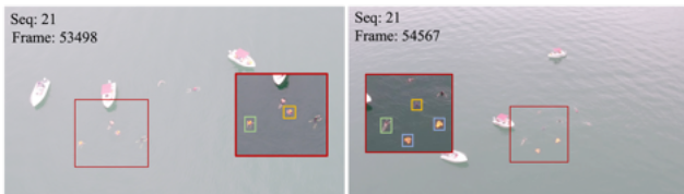
Figure 4. An example of splitted tracks, in the earlier frame, the swimmers are wearing lifejackets, however, in the later frame, after the lifejackets are taken off, new track ids emerges.
