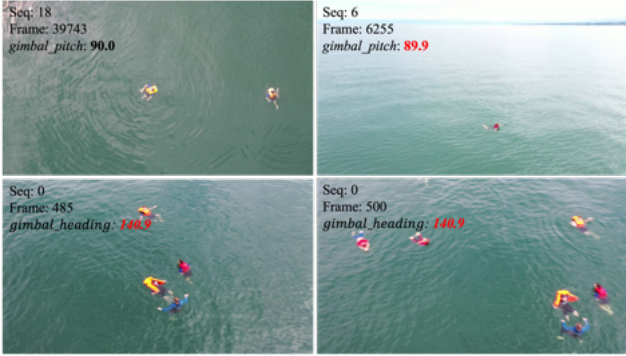
Figure 3. Two types of error in our final results. Top row: Example of gimbal pitch error in the metadata found in the testing split. The two frames have nearly identical pitch, but the drone’s directions are clearly different. Bottom row: Example of the metadata is not synchronized with the actual drone gimbal.
