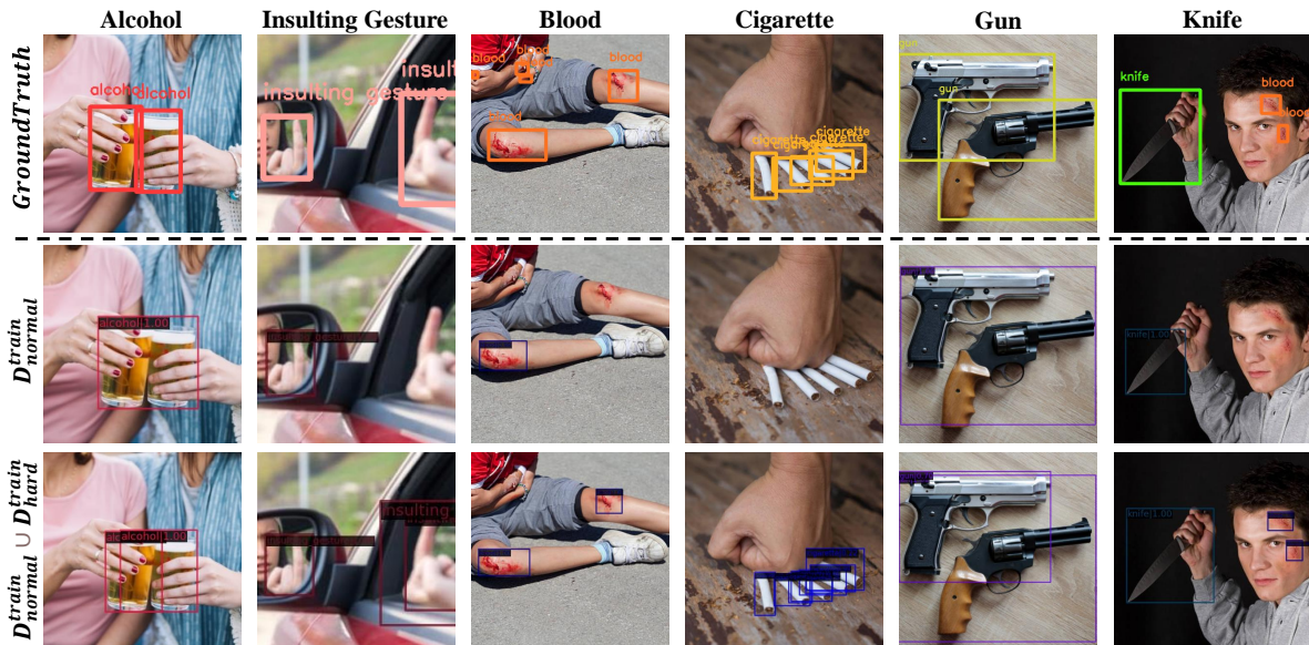
Figure 3. The example images from our hard case test dataset and the corresponding inference results. The first row represents hard case ground-truth samples from the dataset \mathcal{D}_{hard}^{test} . The second row shows the detection results using Faster R-CNN trained on only \mathcal{D}_{normal}^{train} . The third row represents the detection results using Faster R-CNN trained on the joint dataset \mathcal{D}_{normal}^{train} \cup \mathcal{D}_{hard}^{train} . We have found hard case training images can greatly improve the detection models’ robustness.
