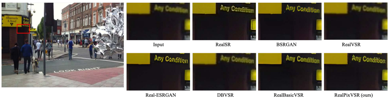
Figure 3. Qualitative Comparison [Clip 13 - Frame 10] . The proposed RealPixVSR effectively uses the pixel-level degradation representation and its recurrent propagation to super-resolve images with more detail compared to other models.
