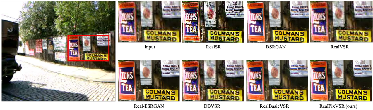
Figure 10. Qualitative Comparison [Clip 37 - Frame 98] . The proposed RealPixVSR effectively uses the pixel-level degradation representation and its recurrent propagation to super-resolve images with more detail compared to other models.
