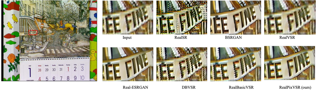
Figure 9. Qualitative Comparison [Clip 30 - Frame 20] . The proposed RealPixVSR effectively uses the pixel-level degradation representation and its recurrent propagation to super-resolve images with more detail compared to other models.
