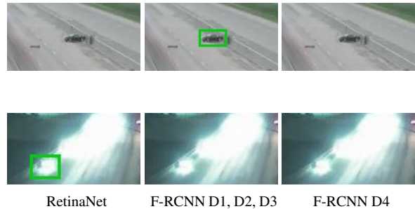
Figure 10. Our Faster RCNN detectors can detect cars from many angles including side-angle whereas other models cannot. RetinaNet detector is capable of detecting cars from night scenes, which are extremely hard detection.
