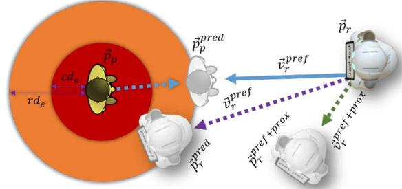
**Figure 5:** Our robot navigation algorithm satisfies the proxemic distance constraints, including peripersonal space (green) and interpersonal space (blue). The trajectory computed by our algorithm does not intrude onto these spaces, whereas a robot that fails to consider the reachability distance (purple trajectory) may cause discomfort to some pedestrians.
