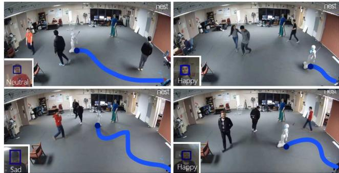
**Figure 1:** We present a real-time data-driven planning algorithm that learns about pedestrians' emotional state in order to navigate socially aware. The robot learns in real time about the emotions of pedestrians and their proxemic constraints. These distances limit the movement and navigation of the robot to avoid intrusion into peripersonal and interpersonal social spaces of the pedestrian. Combining emotional and proxemic constraints enhances social comfort as well as navigation.
