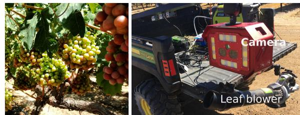
Figure 2. *Left*: Closeup view of the vineyard. *Right* Imaging equipment with camera and air blower
