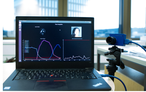
Figure 3. The demonstration setup involving a DVS sensor providing input to the SINABS to simulate a multi-layer SCNN.
