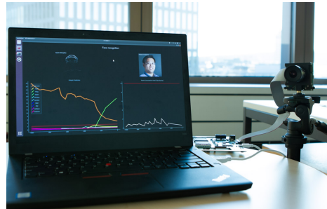
Figure 4. In this demonstration setup, a DynapCNN receives input directly from a DVS.
