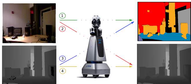
Figure 1. Scenarios for RGB-D data include semantic segmentation from RGB (1), depth (3) or both (1+3), depth prediction from RGB (2) and depth completion from depth (4).
