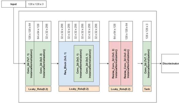
Figure 1. Structure of the Generator network
