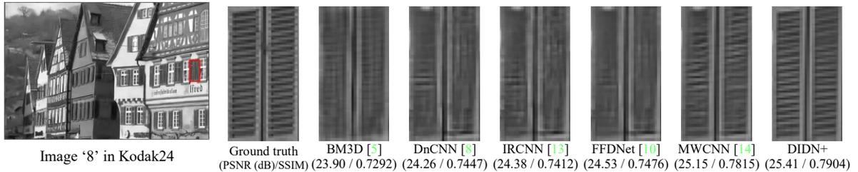
Figure 5: Grayscale image denoising results at noise level 50.
