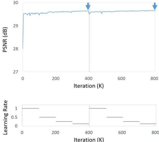
Figure 4: Weight averaging points. Upper and lower t indicate validation PSNR (dB) and learning rate, respectively, during training.
