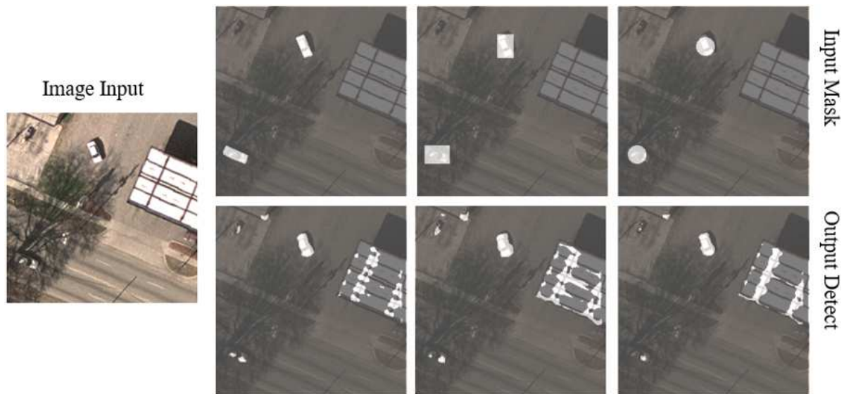
Figure 7. Example of each networks output detection with an occluded target and a significant false positive detection. From left to right, the polygon network, bounding box network, and point target network. Input Image courtesy of the U.S. Geological Survey.
