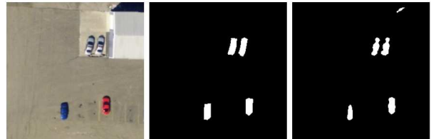
Figure 3. Example of, from left to right, an input image from OIRDS, a polygon input mask, and the output of the trained network for reference. See Figure 6 and 7 for input masks and outputs for the bounding boxes and point targets. Input Image (left) courtesy of the U.S. Geological Survey.
