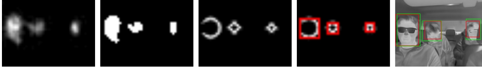
Figure 5. Stages of splitting the heatmap to connected regions and applying blob detection to get the enclosing bounding boxes.
