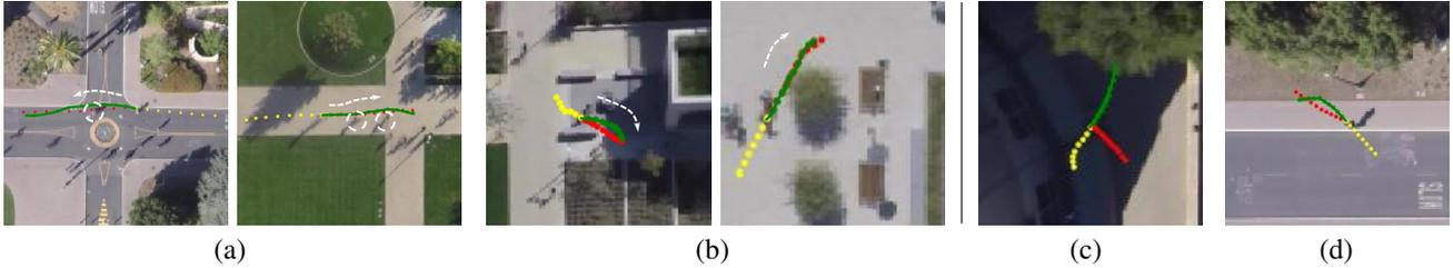
Figure 4: Qualitative evaluation. (Color codes: Yellow - given past trajectory, Red - ground-truth, and Green - our prediction)
