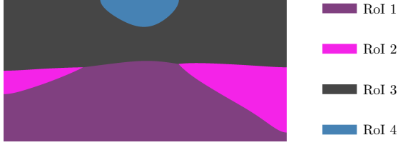
Figure 4. Regions of interest derived from the priors of the classes building, road, sidewalk and sky in the Cityscapes dataset.
