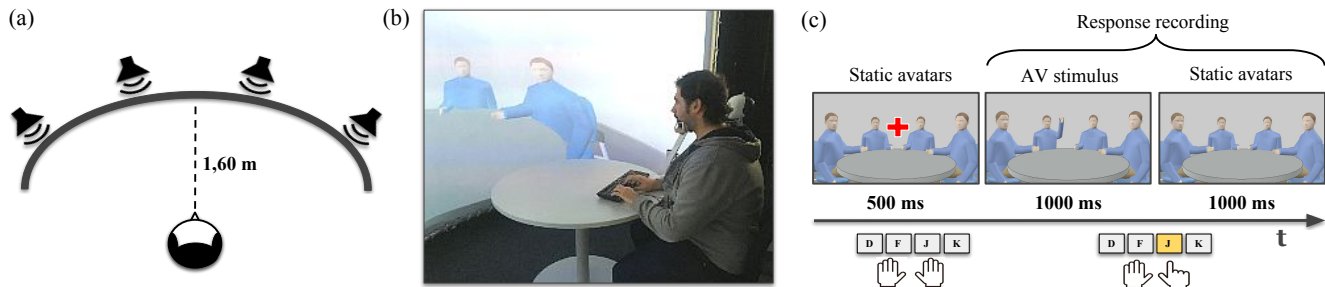
Figure 1: Behavioural study on audio-visual localization: (a) Immersive experimental setup with acoustically transparent concave projection screen (b) Subject selecting a position via a keyboard (c) Schematic illustration of one trial of the AV localization task.
