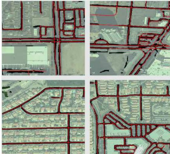
Figure 3. Four sample predictions in Las Vegas from the model trained in Las Vegas. Background shows the input imagery overlaid with the shaded road predictions from the model and red lines show the labels.
