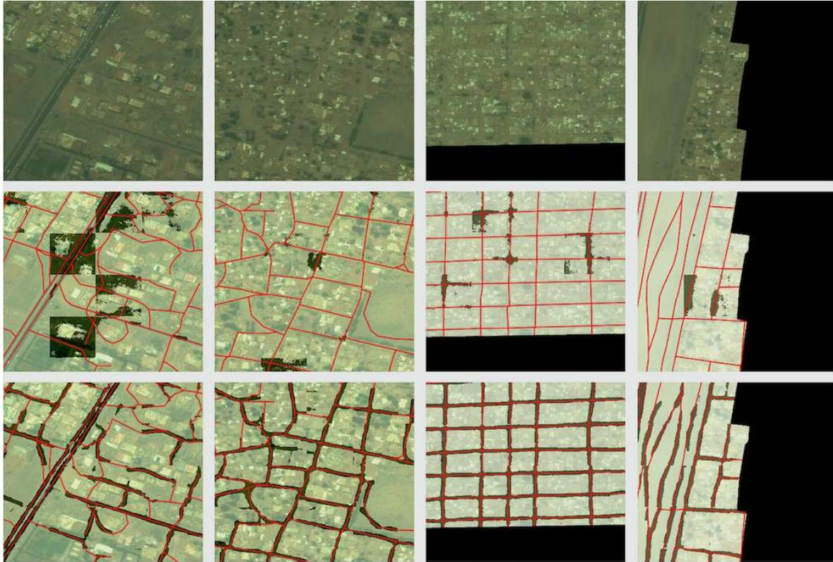
Figure 4. Prediction results in Khartoum for four different scenes. Top: input imagery, middle: prediction results (shaded) from the model trained in Las Vegas overlaid with labels (red lines) on top of the input imagery, bottom: prediction results (shaded) from the model trained in Khartoum overlaid with labels (red lines) on top of the input imagery.
