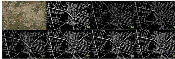
Figure 1. Comparison of NN Models. An example (a) satellite image and (b) ground truth; and road predictions using (c) VGG; (d) U-Net; (e) ResNet50; (f) ResNet101; (g) SegNet; and (h) DeepLab (source: [10]).
