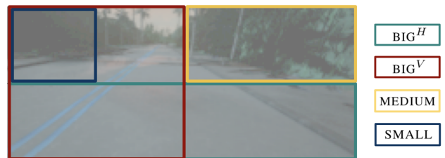
Figure 3: Four sliding windows are used to generate a multi-scale grid of RoIs. Colors indicate the box type: BIG V (red), BIG H (green), MEDIUM (yellow) SMALL (blue).
