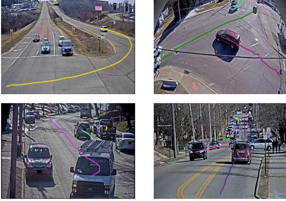
Figure 3. Motion paths generated from the centers of vehicles.
