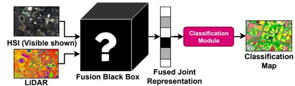
Figure 1. Generic schematic of a multimodal fusion based classification task. The objective is to effectively combine the two modalities (hereby HSI and LiDAR) such that the resultant representation has rich, fused features that are relevant and robust enough for accurate classification.
