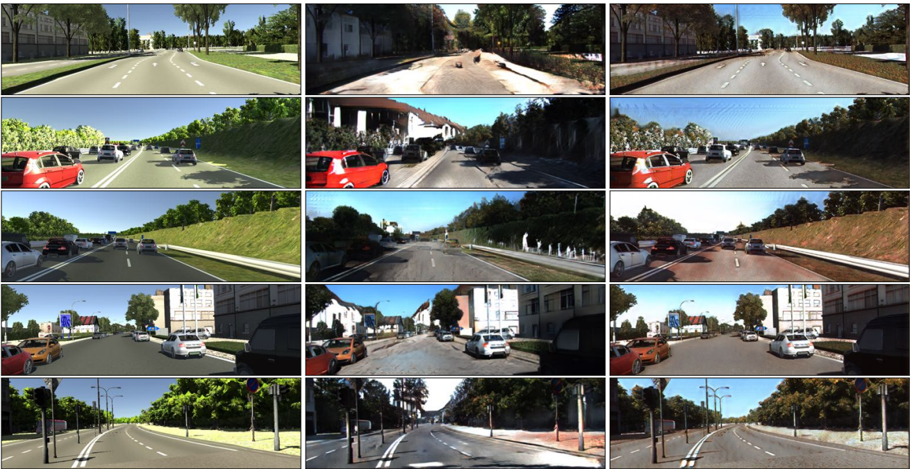
Figure 4. Qualitative results on input-level adaptation. From left to right: left: input synthetic image, we compare the image translation results of middle: CycleGAN, with right: GIO-Ada result. Note that CycleGAN hallucinates objects in the transformation process, while GIO-Ada is able to preserve the semantic and geometric information.
