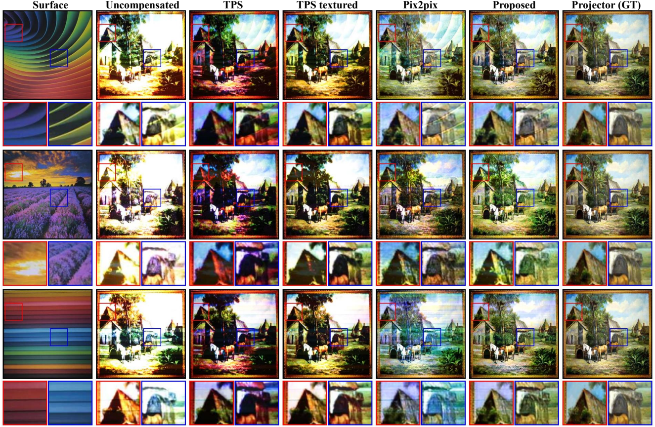
Figure 4: Comparison of TPS [11], TPS textured, pix2pix [18] and CompenNet on different surfaces. The 1 st column is the camera-captured projection surface. The 2 nd column is the camera-captured uncompensated projected image. The 3 rd to 6 th columns are the camera-captured compensation results of different methods. The last column is the ground truth input image. Each image is provided with two zoomed-in patches for detailed comparison. When trained with diverse textured images, TPS produces better results than its original version [11] that uses plain color images, though still suffers from hard edges, blocky effect and color errors. Compared with CompenNet, pix2pix generates unsmooth pixelated details and color errors.
