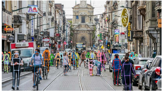
Figure 1: We want to estimate human 2D poses in the transportation domain where autonomous navigation systems operate in crowded scenes. Humans occupy small portion of the images and could partially occlude each other. We show the output of our PifPaf method with colored segments.
