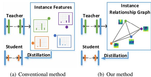
Figure 1: Comparison between the conventional and proposed methods. (a) The conventional method uses instance features to guide the student. Each instance is an independent point in the feature space. (b) The proposed method defines Instance Relationship Graph (containing instance features, instance relationships and feature space transformation) as the distilled knowledge to guide the student.
