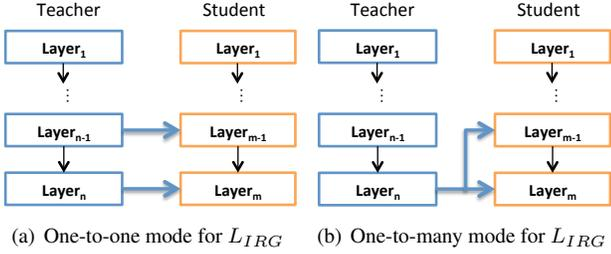
Figure 4: Two possible deploy modes for  $L_{IRG}$ .
