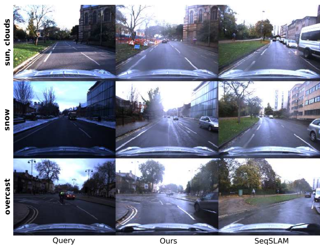
Figure 7. Visual examples of our method correctly localizing, while SeqSLAM baseline fails on Oxford Robotcar dataset.
