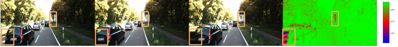
Figure 1: Left to right: left image, right image, left reconstruction, adaptive weights. The adaptive weights reduce regularization at regions of high residual; hence, they discount dis-occlusions and occlusions as in the highlighted regions.
