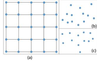
Figure 1. **Image grid vs. point cloud.** (a) shows a  $5 \times 5$  local region in a image, where the distance between points can only attain very few discrete values; (b) and (c) show that in different local regions within a point cloud, the order and the relative positions can be very different.
