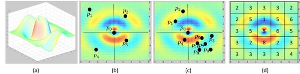
Figure 2. **2D weight function for PointConv.** (a) is a learned continuous weight function; (b) and (c) are different local regions in a 2d point cloud. Given 2d points, we can obtain the weights at particular locations. The same applies to 3D points. The regular discrete 2D convolution can be viewed as a discretization of the continuous convolution weight function, as in (d).
