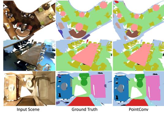
Figure 7. **Examples of semantic scene labeling.** The images from left to right are the input scenes, the ground truth segmentation, and the prediction from PointConv. For better visualization, the point clouds are converted into mesh format. Best viewed in color.
