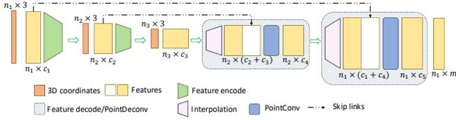
Figure 4. **Feature encoding and propagation**. This figure shows how the features are encoded and propagated in the network for a  $m$  classes segmentation task.  $n$  is the number of points in each layer,  $c$  is the channel size for the features. Best viewed in color.
