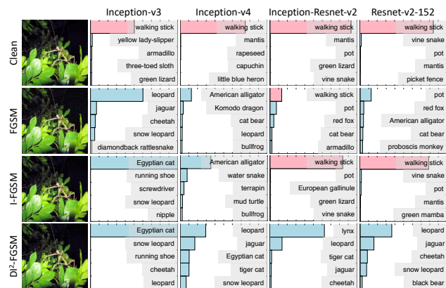
Figure 1. The comparison of success rates using three different attacks. The ground-truth “walking stick” is marked as pink in the top-5 confidence distribution plots. The adversarial examples are crafted on Inception-v3 with the maximum perturbation \epsilon = 15 . From the first row to the the third row, we plot the top-5 confidence distributions of clean images, FGSM and I-FGSM, respectively. The fourth row shows the result of the proposed Diverse Inputs Iterative Fast Gradient Sign Method (DI 2 -FGSM), which attacks the white-box model and all black-box models successfully.
