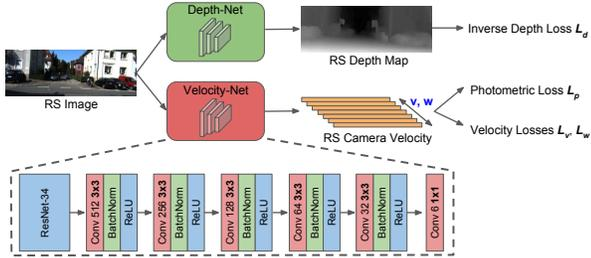
Figure 3. Detailed architecture of our structure-and-motion-aware RS correction network.
