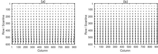
Figure 5. Resemblance between: (a) undistortion flow required to compensate the distortion introduced by RS camera rotation  $w_x$  and (b) vertical image resizing, confuses network training.
