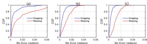
Figure 6. Performances of our networks when trained with cropped images or resized images and tested on image sets with: (a)  $w_x$ -rotation only, (b)  $w_y$ -rotation only, and (c)  $w_z$ -rotation only.
