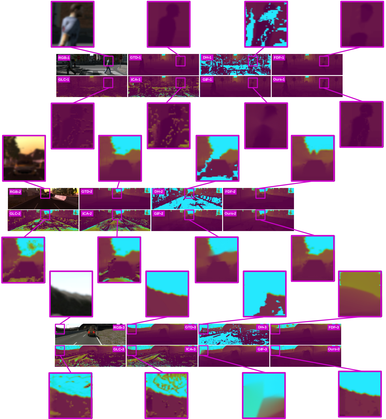
Figure 8: Comparison of depth completion methods applied to synthetic test set. RGB : input colour image; GTD : Ground Truth Depth; DH : Depth Holes; FDF : Fourier based Depth Filling [1]; GTS : Global and Local Completion [7]; ICA : Inpainting with Contextual Attention [12]; GIF : Guided Inpainting and Filtering [9].
