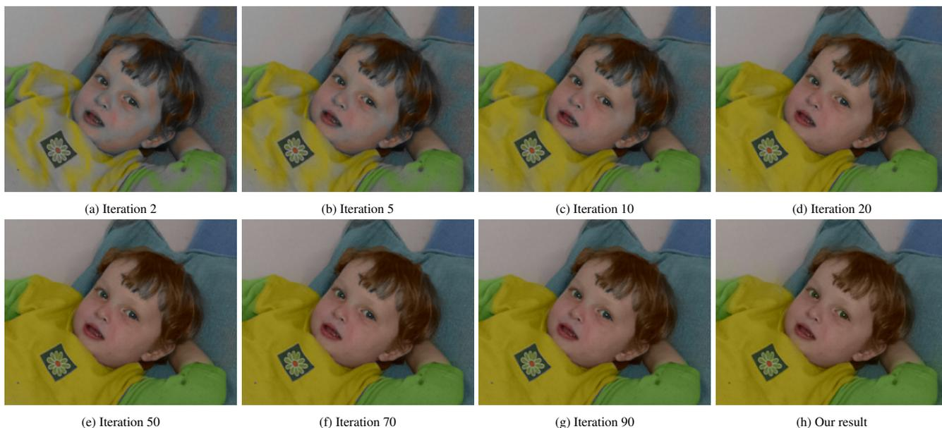
Figure 3: Propagation of colors: (a-h) shows how the colors from the user-annotated strokes propagate through the image while not crossing strong image edges using DTS. After iteration 50, the changes are small and can be ignored as a trade-off for speed.
