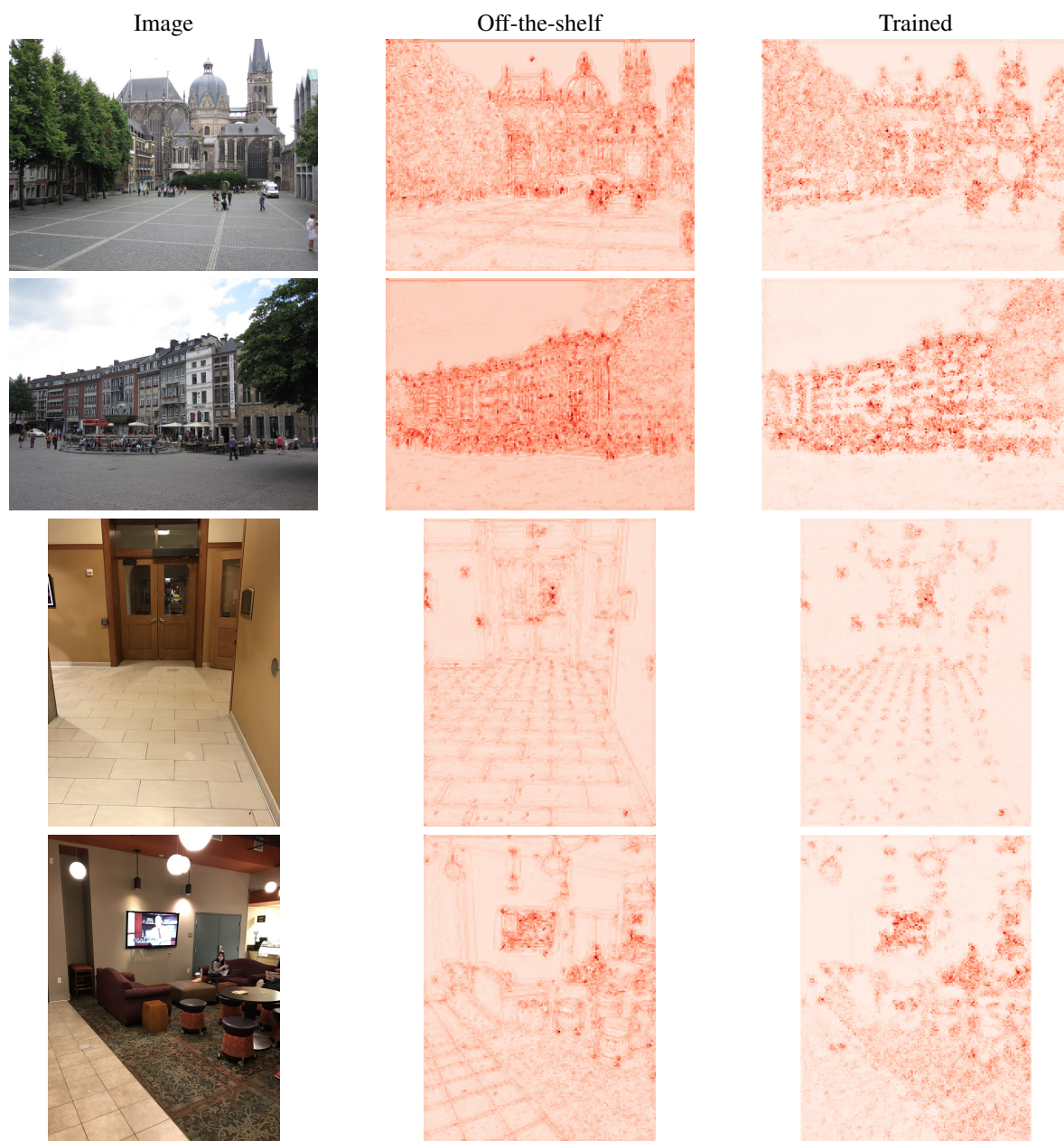
Figure 4: Soft detection scores for different scenes before and after fine-tuning. White represents low soft-detection scores while red signifies higher ones. The training lowers the soft-detection scores on repetitive structures ( e.g. ground, floor, walls) while it enhances the score on more distinctive points. This is shown by the increased contrast of the trained soft-detection maps with respect to their off-the-shelf counterparts.
