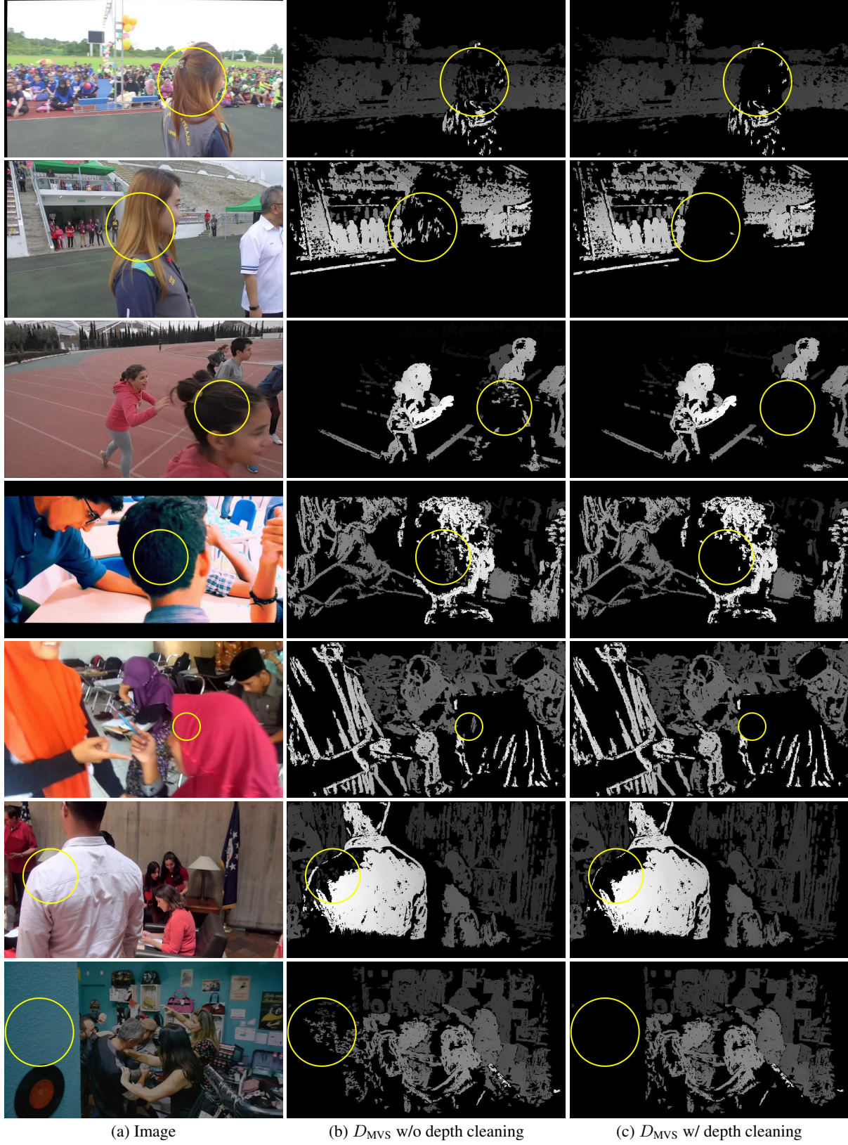
Figure 4: Effects of proposed depth cleaning method. See regions circled in yellow. Proposed depth cleaning method using Eq. (1) in our main paper removes outliers of MVS depth D_{MVS} significantly.
