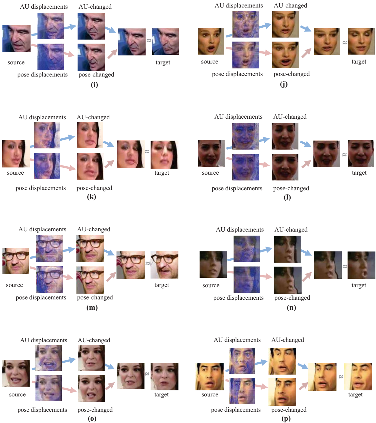
Figure 1. Visualizations of the pose and AU transforms for 16 subjects. The source is transformed to the AU-changed and pose-changed face images through the AU displacements and pose displacements respectively. AU-changed face image should have the same AUs as the target and the same pose as the source. Pose-changed face image should have the same pose as the target and the same AUs as the source. Better viewed in color and zoom in.
