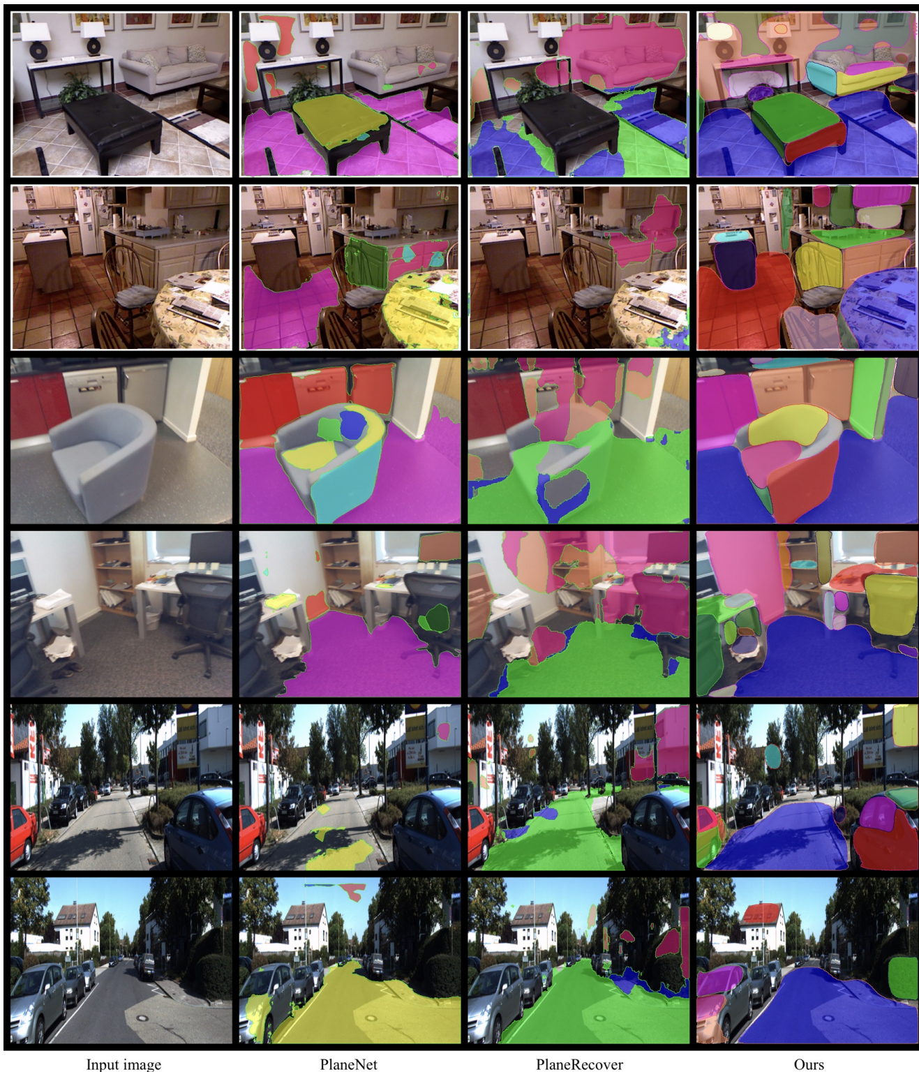
Figure 4. More plane segmentation results on unseen datasets without fine-tuning. From left to right: input image, PlaneNet [5] results, PlaneRecover [10] results, and ours. From top to the bottom, we show two examples from each dataset in the order of NYUv2 [9], 7-scenes [8], and KITTI [1].
