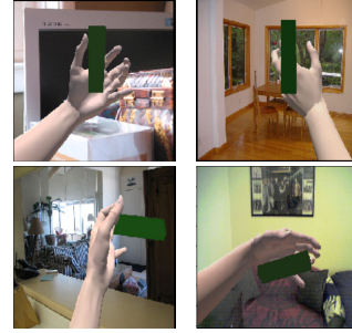
Figure 1: We extract the foreground objects in our training images and composite them over random images from PASCAL VOC [1]. We also augment the training set by superimposing segmentation masks of objects of interest for which the 6D poses are known to be able to simultaneously predict the hand and object pose and gain robustness against object occlusions.
