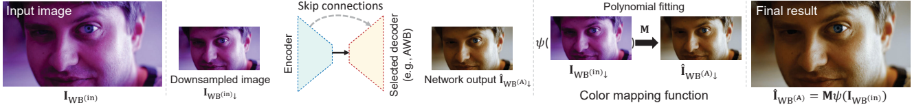
Figure 3: We consider the runtime performance of our method to be able to run on limited computing resources ( \sim 1.5 seconds on a single CPU to process a 12-megapixel image). First, our DNN processes a downsampled version of the input image, and then we apply a global color mapping to produce the output image in its original resolution. The shown input image is rendered from the MIT-Adobe FiveK dataset [11].
