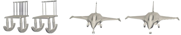
Figure 9: Failure in capturing thin structures. In each pair: ground truth model (left), and SAL reconstruction (right).
