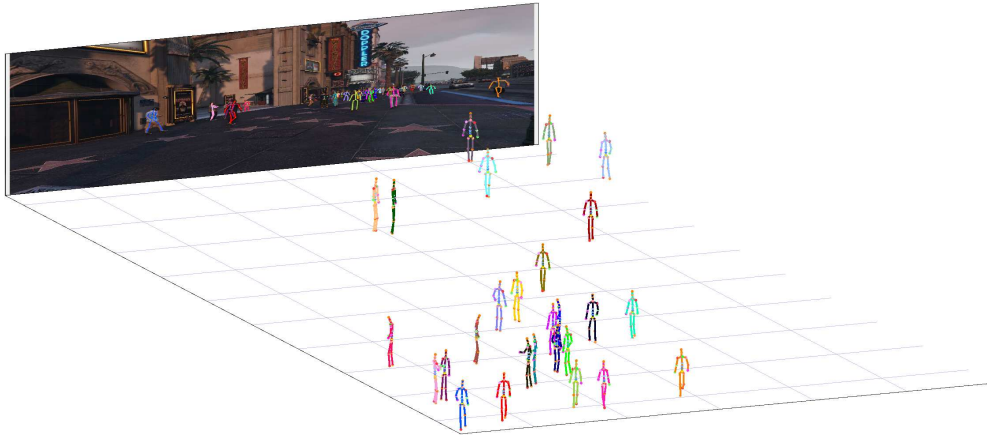
Figure 1: Qualitative results of PandaNet on JTA dataset [8] which consists in images with many people (up to 60), a large proportion of people at low resolution and many occlusion situations. Most of the previous 3D human pose estimation studies mainly focused on the single-person case or estimate 3D pose of few people at high resolution. In this paper, we propose an anchor-based and single-shot multi-person 3D pose estimation framework that allows the pose estimation of a large number of people at low resolution. Ground-truth translations and scales are used for visualisation.
