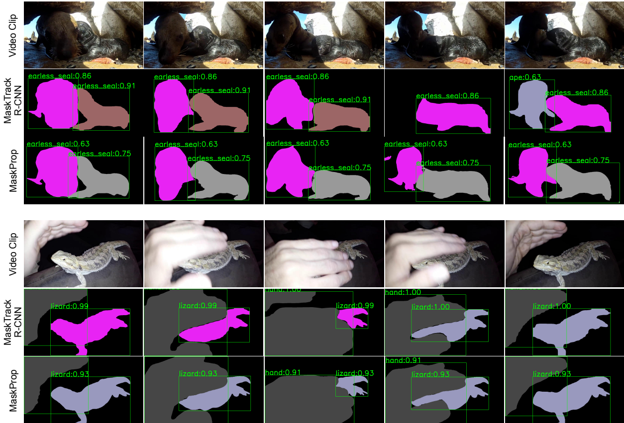
Figure 7: We compare our video instance segmentation results with MaskTrack R-CNN [42] predictions. Different object instances are encoded with different colors. The first row for each video shows the original frames. The second row illustrates the mask predictions of MaskTrack R-CNN and the third row those obtained with our MaskProp. Compared to MaskTrack R-CNN, our MaskProp tracks object instances more robustly even when they are occluded or overlap with each other. Additional video instance segmentations produced by our method are included in our supplementary video 1 .
