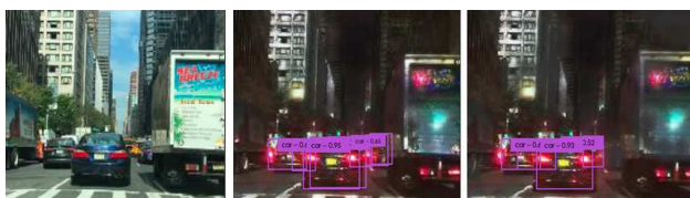
Figure 7: Predicted detections for an input day image (left) using RetinaNet (middle), Faster-RCNN (right). Note that the higher mAP of RetinaNet yields better instance translations.
