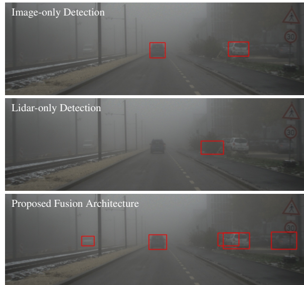
Figure 1: Existing object detection methods, including efficient Single-Shot detectors (SSD) [41], are trained on automotive datasets that are biased towards good weather conditions [19, 59], they fail in rare weather events (top). Lidar-only detectors, such as the same SSD model trained on projected lidar depth, might be distorted due to severe backscatter in fog or snow (center). These asymmetric distortions are a challenge for fusion methods, that rely on redundant information. The proposed method (bottom) learns to tackle unseen (potentially asymmetric) distortions in multimodal data without seeing training data of these rare scenarios.
