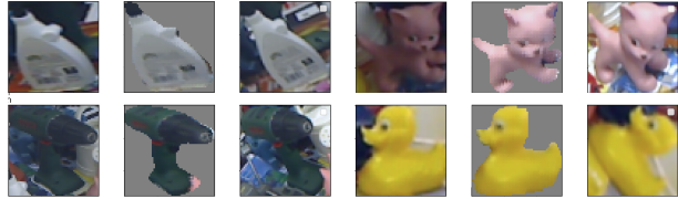
Figure 7. The reconstruction (middle) of the source (left) by warping the target (right) using matched landmark positions.
